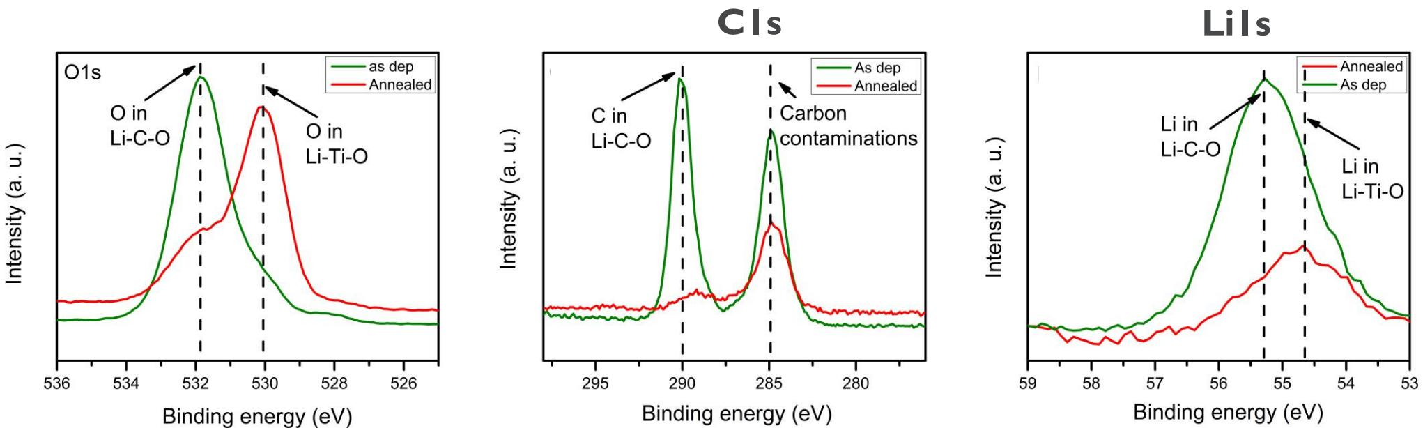
The thermal treatment causes elements intermixing and the LTO material formation
