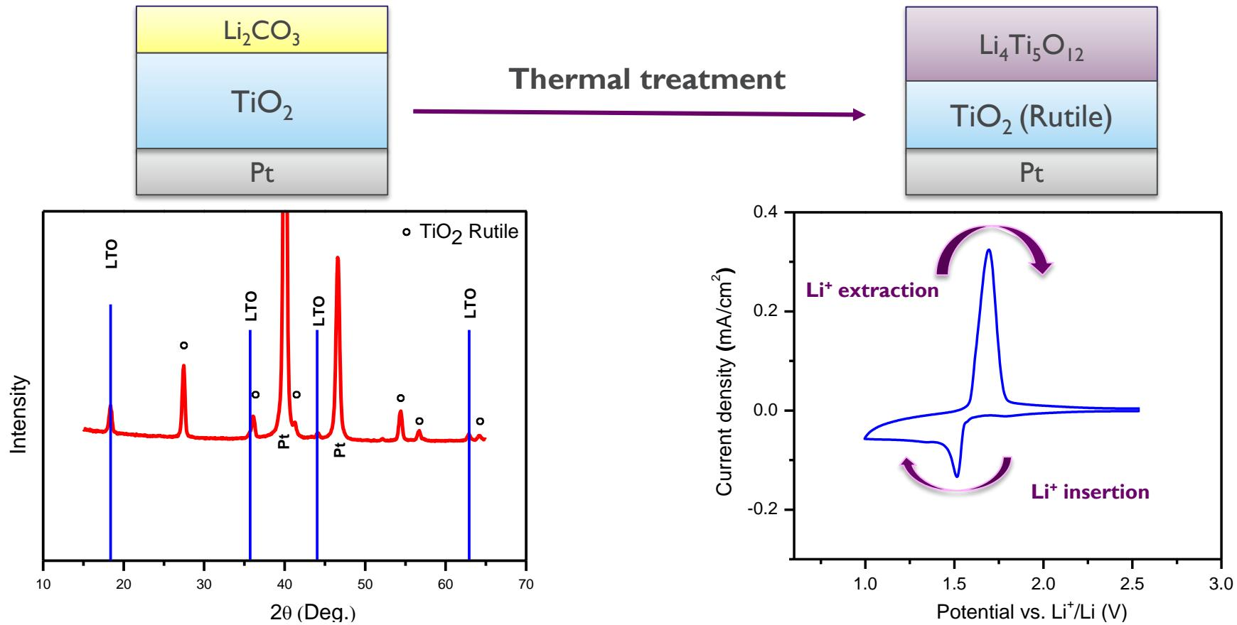
Spinel LTO diffraction peaks together with rutile  $\text{TiO}_2$  and Pt substrate peaks
