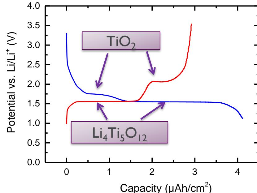
Redox peaks attributed to  $\text{Li}_4\text{Ti}_5\text{O}_{12}$  and  $\text{TiO}_2$
