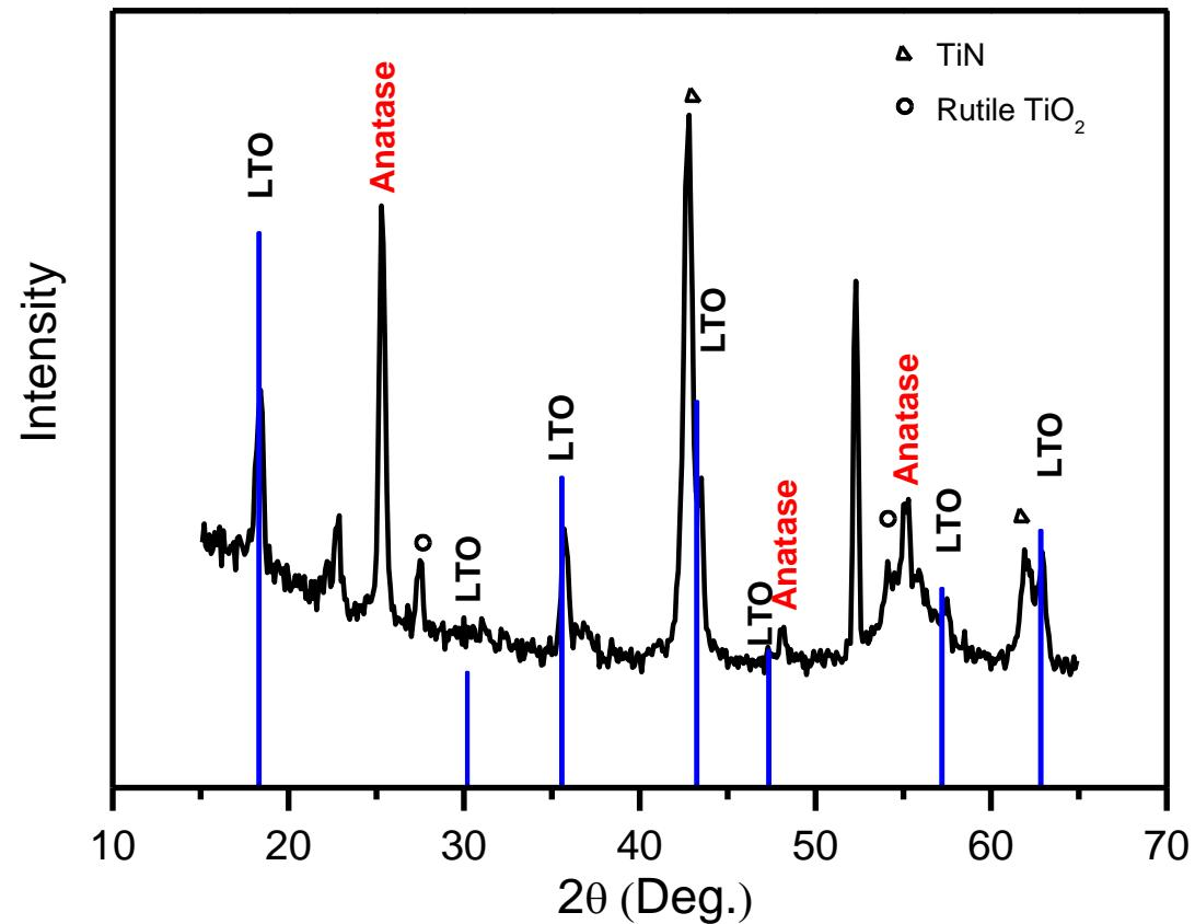
Characteristic spinel LTO diffraction peaks together with  $\text{TiO}_2$  (mainly anatase and some rutile) and TiN current collector peaks.
