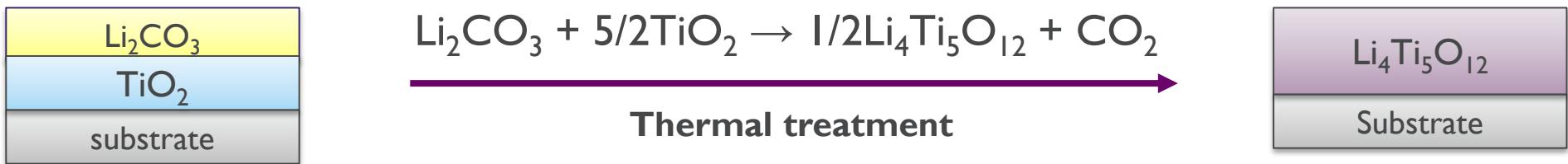
The  $\text{TiO}_2$  layer is deposited by sputtering or atomic layer deposition (ALD)
