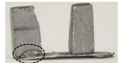
Brazing materials incompatibility - Reaction zone
